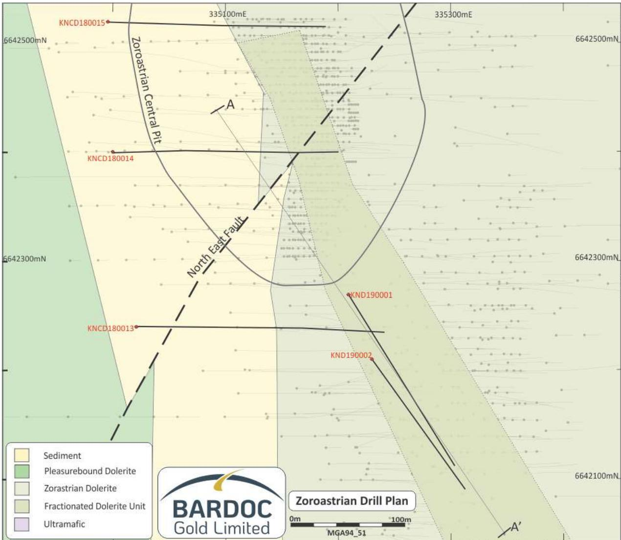
**Figure 1: Zoroastrian Plan View showing recent drilling locations. Note drill orientation of KND190001 and KND190002 designed to remain within the favourable host dolerite unit**
